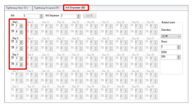
**Step 2:** After setting parameters to Program 1 in Tightening Program (TP), then click button to save the data to the controller.
