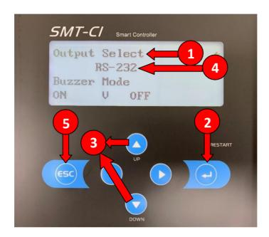
**NOTE:** This is **RS-232** (flashing light indicates successful connection).
