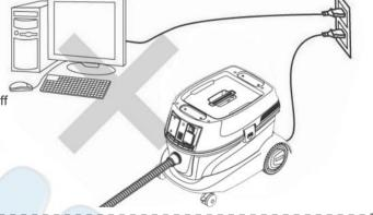
Avoid to twist, bend, trample on, pull, forced the hose and unusual storage to make it out of shape and cause damage.
