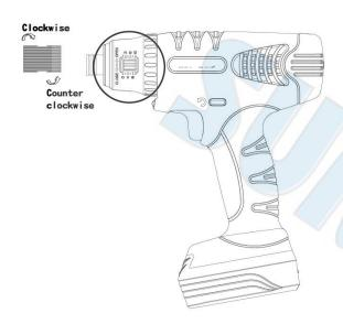
(1)Remove the torque cover by turning it counterclockwise.
