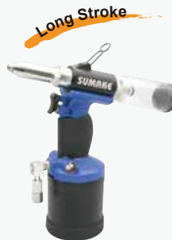
ST-66165V Vacuum ST-66165N Non-vacuum 3/16" (4.8mm)
