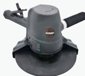
ST-7789 9" Industrial vertical grinder Side Exhaust Speed: 6,500 rpm Spindle: M16x2.0
