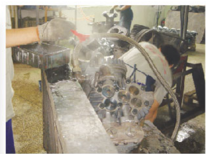
Air Leakage Test
