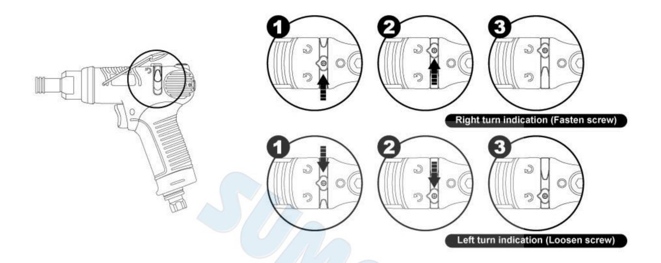
Bit convert operation of Pull type tool
