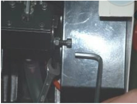
Screw delivery air volume adjustment
