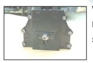
WHEN TOP EDGE OF ADJUSTMENT PLATE (019) IS AT IT'S HIGHEST SETTING(NO.4), THE TEETH(021,022) ARE AT THEIR SHALLOWEST PENETRATION. IF SET AT LOWEST SETTING (NO,1) THE TEETH (021,022) ARE AT THEIR DEEPEST PENETRATION.
