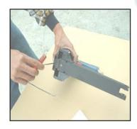
LOOSEN SET SCRCW (526) WITH 3 mm HEXAGON WRENCH KEY.
