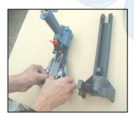
SLIDE LINKAGE MECHANISM AND ADJUSTING ROD (018) SIMULTANEOUSLY FROM COLLAR (006).
