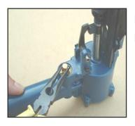
REMOVE VALVE (017) AND TUBE (016) WITH A LONG NOSE PLIERS .
