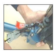
REMOVE SPRING (012) LONG NOSE PLIERS.
