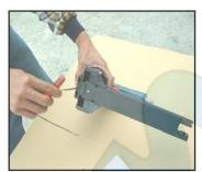
LOOSEN SET SCREW (526) WITH 3  ${\rm mm}$  HEXAGON WRENCH KEY TO UNLOCK ADJUSTING ROD (018) .
