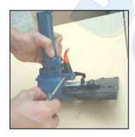
LOOSEN SCREWS (513) WITH FLAT SCREW DRIVER.
