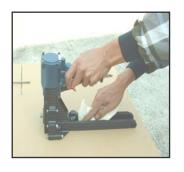
REMOVE TAR BUILDUP WITH KEROSENE #2 FUEL OIL OR DIESEL FUEL . DO NOT ALLOW SOLVENT TO GET INTO THE CYLINDER OR DAMAGE MAY OCCUR . DRY OFF THE TOOL COMPLETELY BEFORE USE .
