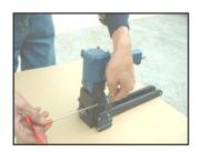
LOOSEN SCREWS (530 , 531) AND NUT (542) WITH 8 mm SPANNER AND 4 mm HEXAGON WRENCH KEY .
