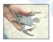
LOOSEN SCREWS (532) WITH 3  ${\rm mm}$  HEXAGON WREM KEY . CHANGE TEETH ONE AT A TIME TO PREVENT REVERS TEETH .
