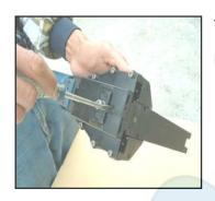
TURN ADJUSTING FOD (018) 180° WITH A SCREW DRIVER TO THE DESIRED ADJUSTMENT.
