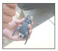
LOOSEN SCREWS (535) WITH 3 mm HEXAGON WRENCH KEY. TAKE OFF THE SPRING PIN (537) WITH HAMMER AND 6 mm STRAIGHT ROD.
