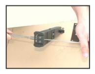
LOOSEN SCREW (539) AND NUT (538) WITH 2.5 mm HEXAGON WRENCH KEY AND 7 mm SOCKET WRENCH.
