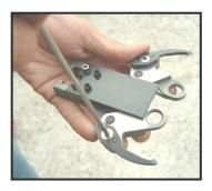
LOOSEN SCREWS (532) WITH 3 mm HEXAGON WRENCH KEY.
