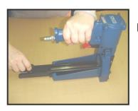
PULL PUSHER (032) BACK UNTIL IT STOPS ON PUSHER PIVOTS (037) THEN ROTATE PUSHER (032) TO POSITION.
