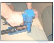
GRASP HANDLE WITH ONE HAND POSITION ON BOX IN LINE WITH THE DESIRED STAPLE LOCATION . THERE IS A SMALL PROJECTION EITHER SIDE OF THE MAGAZINE SEAT (028) AS AN AID IN LOCATING THE POSITION OF THE STAPLE . (011)
