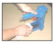
REMOVE TAR BUILD UP WITH KEROSENE #2 FUEL OIL OR DIESEL FUEL . DO NOT ALLOW SOLVENT TO GET INTO THE CYLINDER OR DAMAGE MAY OCCUR . DRY OFF THE TOOL COMPLETELY BEFORE USE .
