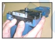
PUSH THE BODY (007) UP AND ADJUST TO DESIRED DEPTH.
