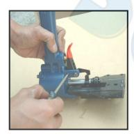
LOOSEN SCREWS (513) WITH FLAT SCREW DRIVER.
