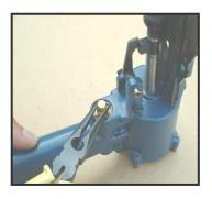
REMOVE VALVE (016) AND TUBE (017) WITH A LONG NOSE PLIER.
