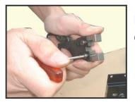
LOOSEN SCREWS (535) WITH 3 mm HEXAGON WRENCH KEY. TAKE OFF THE SPRING PIN (537) WITH HAMMER AND 6 mm STRAIGHT ROD.
