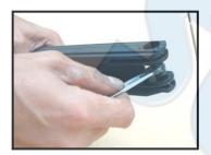
LOOSEN ROD (037) WITH 6 mm OFFSET WRENCH REMOVE PUSHER GUIDES (038). REMOVE PUSHER (032)
