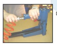
DISCONNECT THE AIR SUPPLY FROM THE TOOL.
