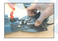
SLIDE LINKAGE MECHANISM AND ADJUSTING ROD (018) SIMULTANEOUSLY FROM COLLAR (006)
