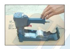
PLACE COIL STAPLES IN MAGAZINE. FEED FRONT END OF COIL STAPLES INTO RIGHT COIL GUIDE (037), LEFT COIL GUIDE (038), AND TOP GUIDE (035). PUSH FORWARD UNTIL STOPPING IN DRIVER GUIDE UNIT (027).
