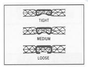
USE ROD(DIA 3 MM) OR 2.5G MM HEXAGON WRENCH KEY. TURN COLLAR (006) THROUGH WINDOW CLOCKWISE TO TIGHTEN CLINCH AND COUNTER-CLOCKVIDE TO LOOSEN CHINCH.
