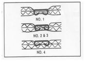
WHEN TOP EDGE OF ADJUSTMENT PLATE (019) IS AT ITS HIGHEST SETTING (NO.4), THE TEETH (021,022) ARE AT THEIR SHALLOWEST PENETRATION. IF SET AT LOWEST SETTING (NO.1) THE TEETH (021,022) ARE AT THEIR DEEPEST PENETRATION.
