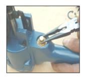
REMOVE VALVE (017) AND TUBE (016) WITH A LONG NOSE PLIERS.
