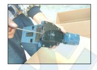
LOOSEN SET SCREW (526) WITH 3 MM HEXAGON WRENCH KEY TO UNLOCK ADJUSTING ROD (018)
