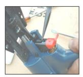
REMOVE SPRING (012) WITH LONG NOSE PLIERS.
