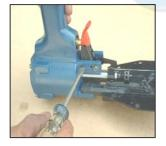
LOOSEN SCREWS (513) WITH FLAT SCREW DRIVER.
