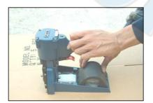
SWING COVER CLOSED AND SLIGHTLY SQUEEZE TO ENGAGE MAGAZINE BOSSES. NOTE : CHECK POSITION ENGAGEMENT.
