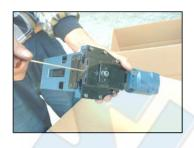
LOOSEN SET SCREW (526) WITH 3 MM HEXAGON WRENCH KEY TO UNLOCK ADJUSTING ROD (018)
