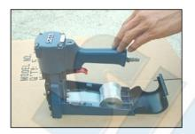
PLACE COIL STAPLES IN MAGAZINE. FEED FRONT END OF COIL STAPLES INTO RIGHT COIL GUIDE (037), LEFT COIL GUIDE (038), AND TOP GUIDE (035). PUSH FORWARD UNTIL STOPPING IN DRIVER GUIDE UNIT (027).
