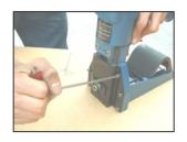
LOOSEN SCREWS (530) WITH 4 MM HEXAGON WRENCH KEY.
