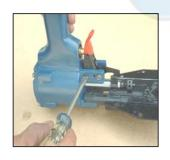
LOOSEN SCREWS (513) WITH FLAT SCREW DRIVER.
