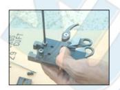
LOOSEN SCREWS (532) WITH 3 MM HEXAGON WRENCH KEY. CHANGE TEETH ONE AT A TIME TO PREVENT REVERS TEETH.
