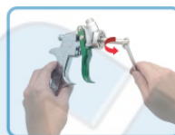
Use 7mm socket to loose Needle Packing Holder with anti-clockwise for changing consumer parts (Needle Packing and SPRING).
