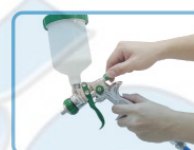
Fluid Control: 1-Small flow: rotate knob with clockwise. 2-Big flow: rotate knob with anti-clockwise.
