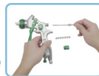
Disassemble knob Fluid Control, to change needle
