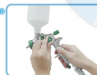
Spray range: 1-Big range: rotate regulation with clockwise. 2-Small range: rotate regulation with anti-clockwise.
