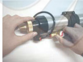
6. First turn 1/3 of red air regulator to spray dust on the work of surface (right now the blue regulator has to be close)
