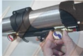
7. According to procedures to do, step by step. If you need bead that will opened the blue regulator to 1/2.
