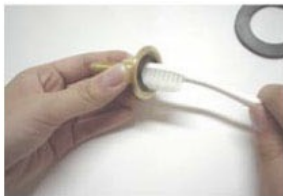
9. If the glue have not dry that can use cleanser and brush to clean. If it had dry that can use knife to shave
