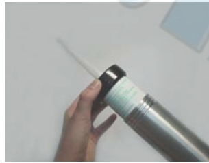
5. Replace Threaded retaining collar on tube
