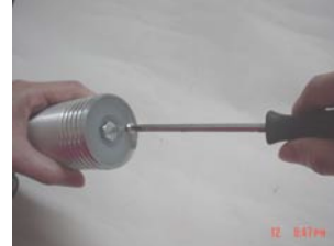
3. Screw out the hole screw
