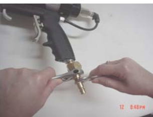
8. Used two wrench to lock nipple
