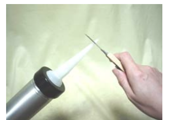
7. Cutting nozzle that you need size
