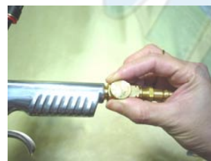
9. Attach air supply to applicator
