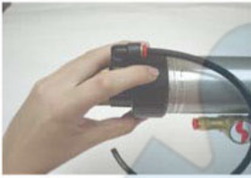
1. First to shift the spray head ass'y
