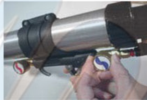
7. According to procedures to do, step by step. If you need bead that will open the blue regulator to 1/2.
