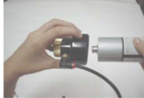
3. Then lock up the glue and spray head ass'y
