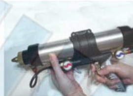
6. Spray out residual glue in tool
