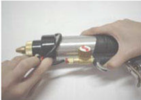
5. plug the air hose into hose jointer
