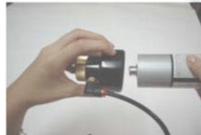
3. Separate the head and glue tube
