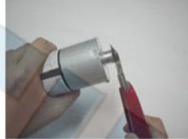
2. Cutting the glue tube head
