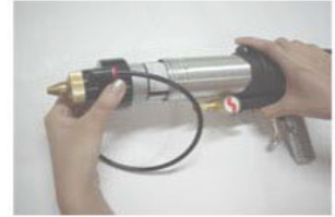
4. put this full ass'y into pipe (If this tool has push rod that will pull it back, if it is line type that will use rod to push piston to button)
