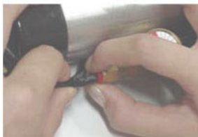
1. First dismantle the air hose
