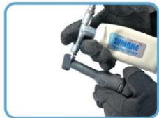
Please add MOLY (Molybdenum Disulfide) grease.
