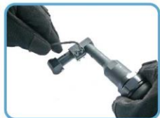
Please add MOLY (Molybdenum Disulfide) grease.
