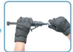
Connect fitting with the air hose.
