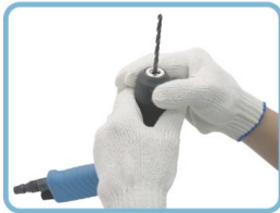
Holding the underneath piece of chuck and then clockwise the above piece in order to tighten the drill bit.
