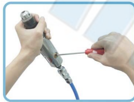
Use slotted screwdriver to adjust speed.
