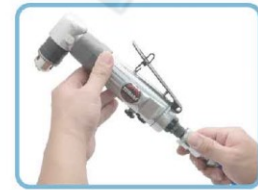
Connect fitting with the air hose.
