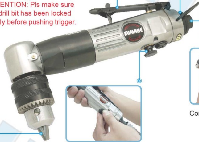
Reverse button: Press the black button along with the trigger on to gets it in a reverse direction. Besides, press and then twist (clockwise) the black one in order to lock in a reverse mode.
