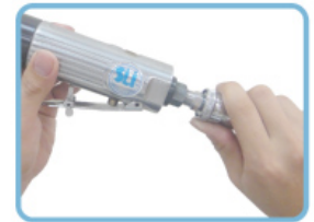
Connect fitting with air hose.
