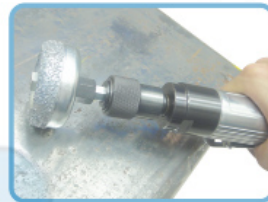
Assembling the metal wheel enable to grind the work piece.
