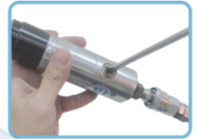
Using a slotted screwdriver to adjust the speed.
