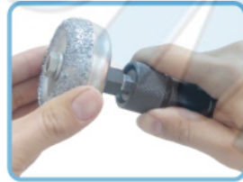
By loosening the quick chuck the adapter would be fixed properly.
