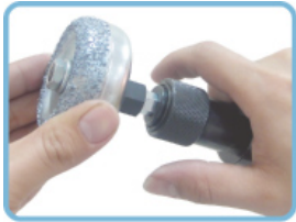
Pulling out the quick chuck and then insert the adapter into the cylinder.
