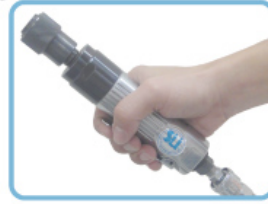
Press the trigger to start the tool.
