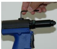
Tighten Oil Plug
