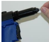
Rivet Head touches Nosepiece
