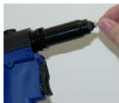
Rivet Head touches Nosepiece
