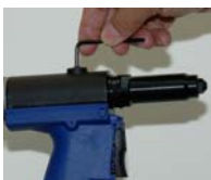
Tighten Oil Plug
