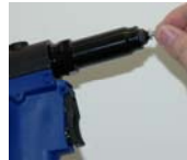
Rivet Head touches Nosepiece
